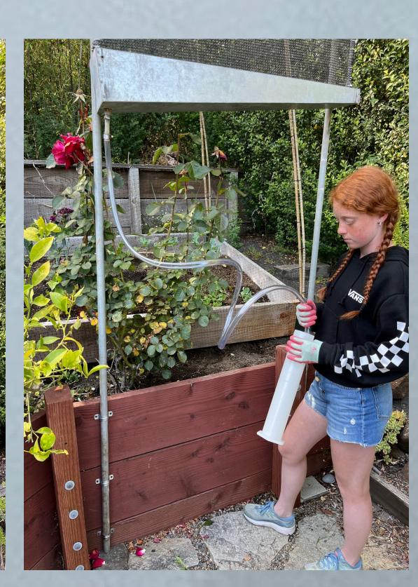
Standard 1.0 m<sup>2</sup> mesh fog collector (windward side of house)
